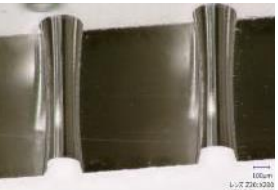
Mirror-finished TGV VIAs developed by NSG
