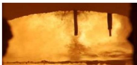
Flame appearance in a furnace with a fuel blend of 80% natural gas and 20% hydrogen.
