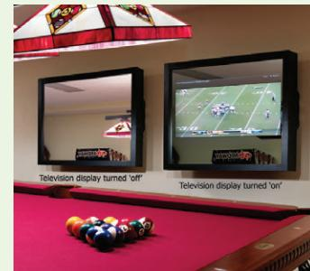
MirroView™ looks like a normal mirror when the screen is 'off'(left). When the screen is 'on,' the image shows through the mirror for a clear view of the screen beneath (right).
